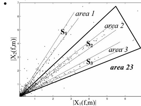
Fig. 3: Scatter-plots of the mixtures at a frequency of 312 Hz for male-male-female combination, a reverberation of 130 ms and a DFT size of 512.
