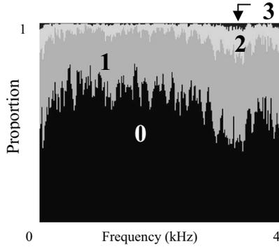
Fig. 1: Histogram of the number of active sources: 0, 1, 2 or 3 for a male-male-female combination recorded with a reverberation of 200 ms and for a DFT size of 512.
