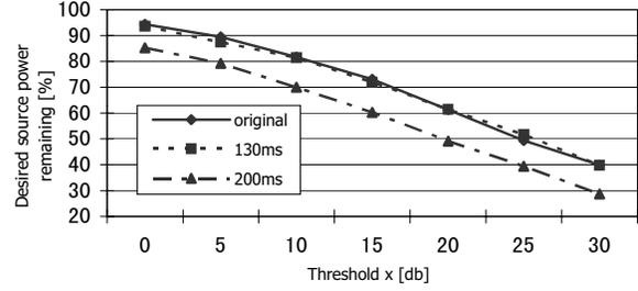
Fig. 2: Approximate WDO against the threshold  $x$  for a DFT size of 512 and a male-male-female combination.
