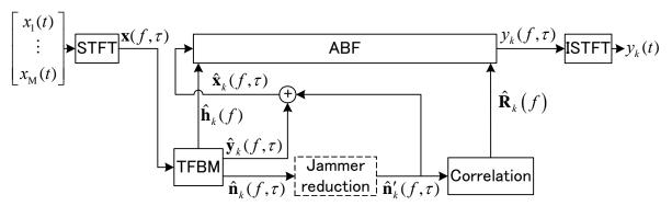
Figure 1: Block diagram of proposed BSS system; ISTFT = inverse STFT.
