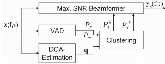
Fig. 2. Block diagram of maximum SNR beamformer
