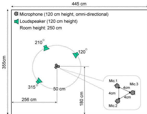
Fig. 5. Recording setup for obtaining room impulse responses
