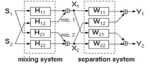
Figure 1. Frequency-domain speech BSS system (N = M = 2)
