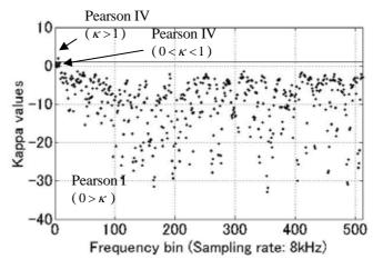
Figure 3.  $\kappa$  values for frequency bin. The horizontal axis indicates frequency bin within 512 STFT frame size and the vertical axis indicates  $\kappa$  value calculated by (9), which was applied to each series obtained by STFT.
