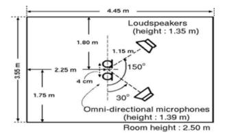
Figure 4. Room layout used for experiments
