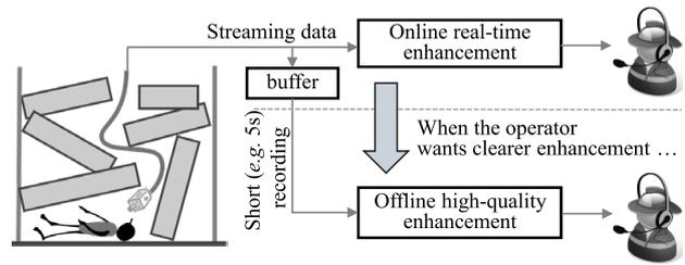
**Fig. 2.** Overview of two-step human-voice enhancement system.
