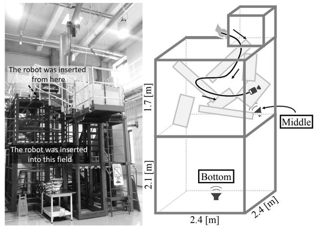
Fig. 8. Mockup rubble field used in Evaluation 1. Two arrangements of the loudspeaker were tested.
