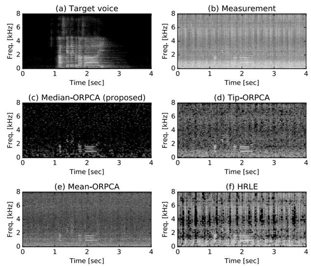
Fig. 10. Examples of online enhancement results obtained when the loudspeaker was at the middle of the field (“Middle”) and the SNR was set to  $-10$  dB. A female voice was emitted between  $1.0$  and  $2.5$  sec.
