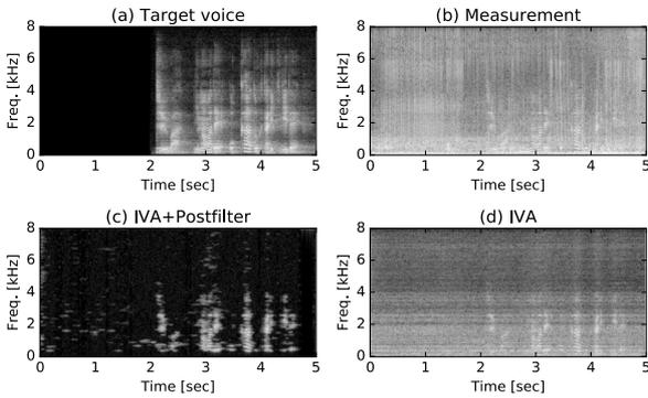
Fig. 12. Examples of offline enhancement results obtained when the loudspeaker was at the middle of the field (“Middle”) and the SNR was set to  $-10$  dB. A male voice was emitted between 2.0 and 5.0 sec.
