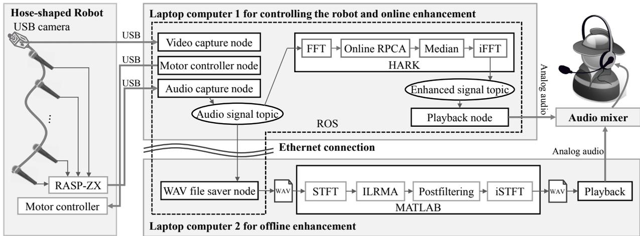
Fig. 7. Configuration of the two-stage human-voice enhancement system.
