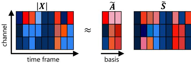
Fig. 1. Time-channel domain representation of observed signals for each frequency bin.
