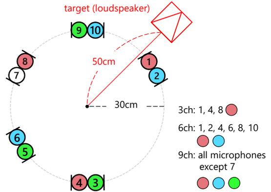
Fig. 3. Arrangement of microphones (IC recorders).
