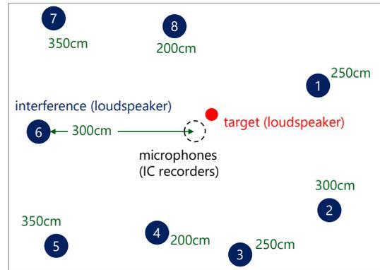
Fig. 2. Arrangement of target, interference sources and microphones.
