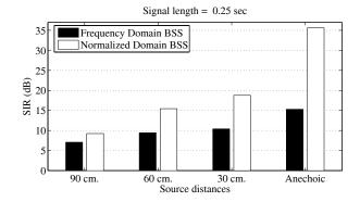
**Fig. 6.** Average SIR gain for sources at different distances. The direct-to-reverberant ratio increases for closer sources. The anechoic situation has infinite direct-to-reverberant ratio. The STFT frame size and number of separation bands were chosen as for Figure 5.
