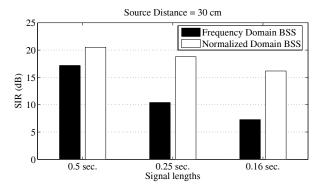
**Fig. 5.** Average SIR gain for different signal lengths. For the normalized BSS one separation band was used. For the FD-BSS the experiments were performed with several different frame sizes, and the sizes which yielded best separation performance were chosen.
