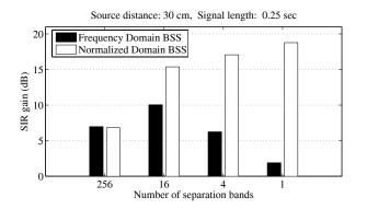
Fig. 4. Average SIR gain for different number of separation bands.
