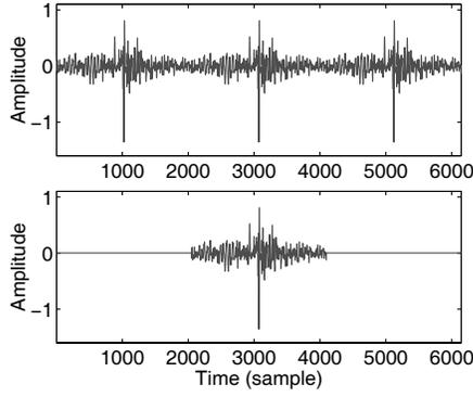
**Fig. 3.** Periodical time-domain filter represented by frequency responses sampled at  $L = 2048$  points (above) and its one-period realization (below).
