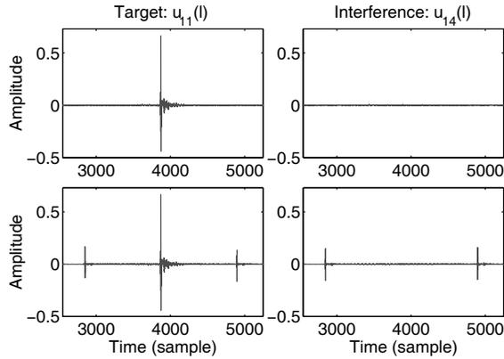
**Fig. 4.** Impulse responses  $u_{ik}(l)$  obtained with the periodical filter (above) and with its one-period realization (below).
