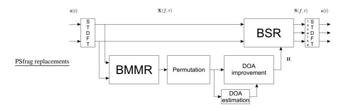
Figure 1: Overall unmixing system
