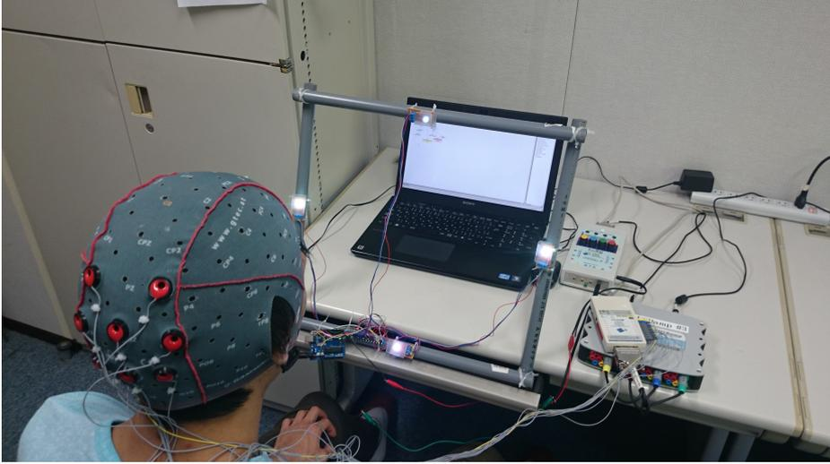
**Fig. 1.** The user seating in front of a frame with four visual stimulation chromatic LEDs used in this study. The picture was included with a permission of the photographed user.
