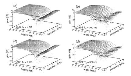
Figure 2: Directivity patterns (a) obtained by BSS ( $T_{\rm R}=0$  ms), (b) obtained by BSS ( $T_{\rm R}=300$  ms), (c) obtained by ABF ( $T_{\rm R}=0$  ms), and (d) obtained by ABF ( $T_{\rm R}=300$  ms).
