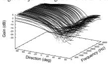
**Fig. 6.** Directivity pattern of separating system obtained by frequency domain ICA
