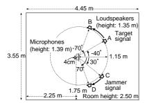
Fig. 3. Layout of room used in experiments.
