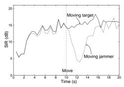
**Fig. 5**. SIR of blockwise batch algorithm without postprocessing. Target and jammer signals moved at 10 sec.
