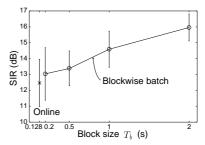
Fig. 4. Average and standard deviation of SIR for fixed sources
