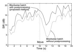
**Fig. 7**. Effect of postprocessing. Jammer signal moved from C to D at 10 sec.
