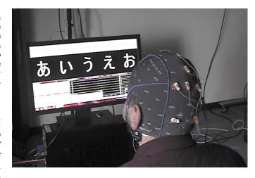
Fig. 1. Visual, auditory and audiovisual BCI speller test paradigm environment based on BCl2000 software [8]. The subject in the picture wears also EEG g.SAHARA electrodes connected to g.MOBllab+ amplifier by g.tec. In this paper we conduct the psychophysical and the preliminary EEG, in offline BCI setting, experiments to evaluate possible differences related to various stimulus perceptions.
