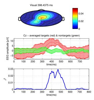
Fig. 7. Visual modality only offline BCI EEG responses presented as scalp mean topography for targets - in the top panel; as the mean time series with standard deviation error-bars for non-targets (green) and targets (red) - in the middle panel; and as the signed statistical difference (i.e., signed  $r^2$ ) value which evaluates the discriminability between the two types of ERPs - in the bottom panel. The figure was created with P300GUI [10].
