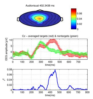
Fig. 8. Audiovisual modality only offline BCI EEG responses presented as scalp mean topography for targets - in the top panel; as the mean time series with standard deviation error–bars for non-targets (green) and targets (red) in the middle panel; and as the signed statistical difference (i.e., signed  $r^2$ ) value which evaluates the discriminability between the two types of ERPs - in the bottom panel. The figure was created with P300GUI [10].
