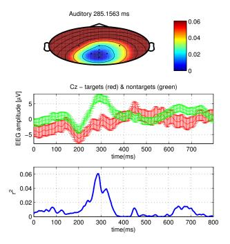
Fig. 6. Auditory modality only offline BCI EEG responses presented as scalp mean topography for targets - in the top panel; as the mean time series with standard deviation error–bars for non-targets (green) and targets (red) in the middle panel; and as the signed statistical difference (i.e., signed  $r^2$ ) value which evaluates the discriminability between the two types of ERPs - in the bottom panel. The figure was created with P300GUI [10].
