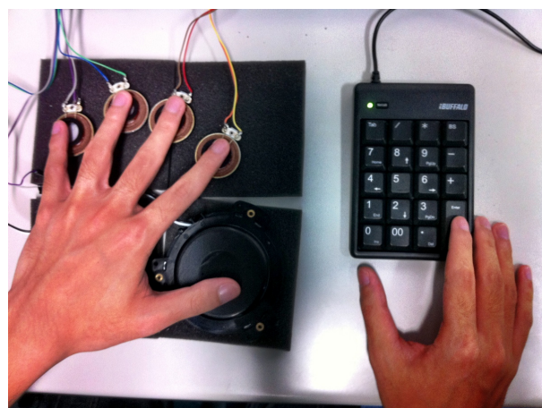
Fig. 1. Vibrotactile stimuli delivered to the left hand finger tips and the palm area using acoustic frequency tactile exciters. The right (dominant) hand is positioned on a response pad used in the psychophysical experiment.
